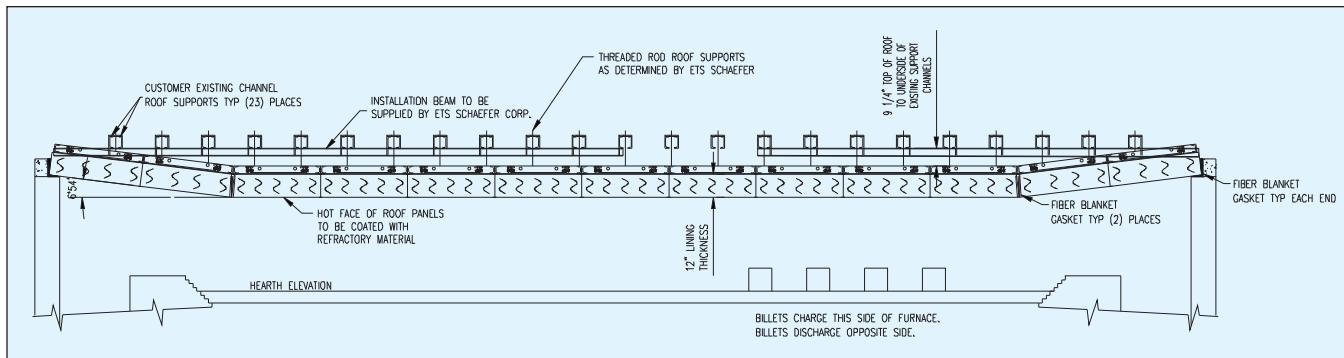
**Fig. 2. AutoCAD drawing of new roof**
